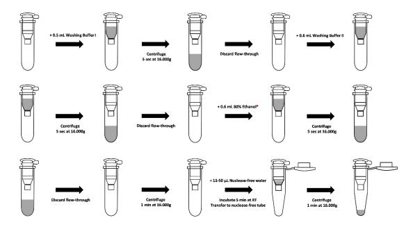
On the final step (iii), the spin column is washed sequentially with Washing Buffer I, Washing Buffer II and 80% ethanol, and the high-quality RNA is eluted in the appropriate volume of RNase-Free Water.
